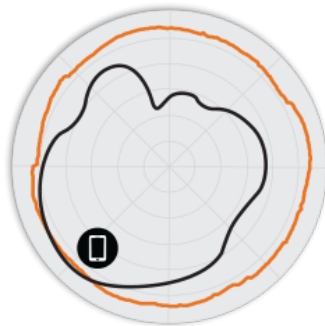
Figure 3. T710o 5GHz Azimuth Antenna Patterns
