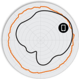
Figure 2. T710o 2.4GHz Azimuth Antenna Patterns
